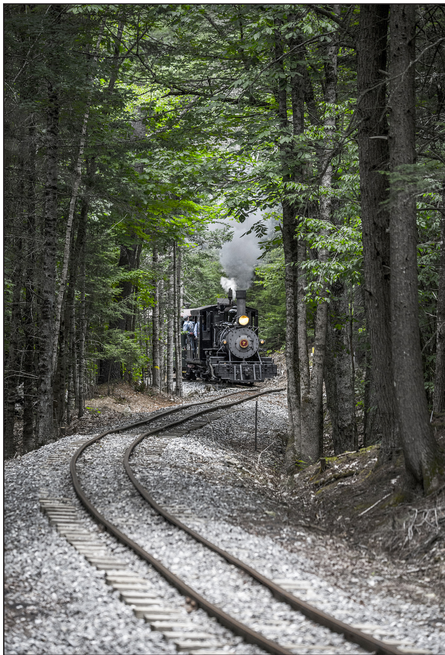
Bridgton & Saco River Baldwin-built 2-4-4 Forney No. 7 attacks the Wiscasset, Waterville and Farmington's 4% grade going from Trout Brook up to Top of Mountain. – Photo © 2019 Dennis Livesey.
