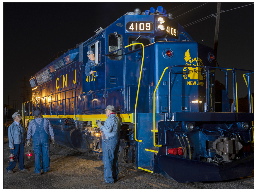
The United Railroad Historical Society's “Museum for a Day” night shoot featured New Jersey Transit's 4109. Originally as CNJ GP40P No. 3677, the latest rebuild made it a GP40PH-2. Recently repainted back to Central Railroad of New Jersey colors, it has proven to be a big hit with employees and fans alike. – Photo © Dennis Livesey.
